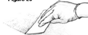
Squeegee away excess epoxy before it begins to gel.
