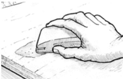
Sand cured fairing compound to desired contour.
